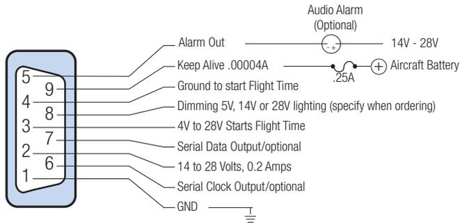
*NOTE: Keep Alive (Pin 9) is only required if alkaline AA size battery is removed. Flight Time starts with either Pin 3 or Pin 4 - use only one pin.*
